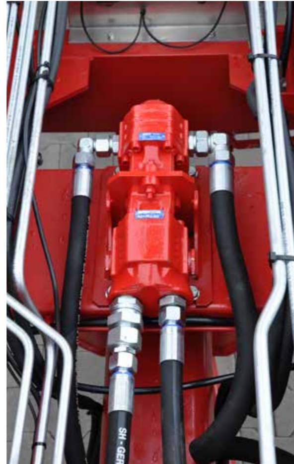
Hydraulic pump driven by an oil engine.
